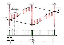
Figure 1: Large momentum transfer interferometric sequence.
